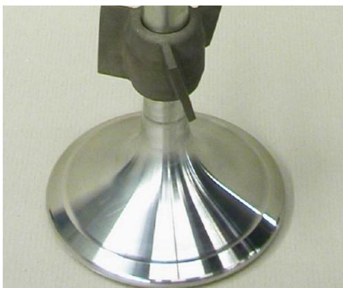
Figure 1. Reconditioned exhaust valve (QuantiServ, 2024).
