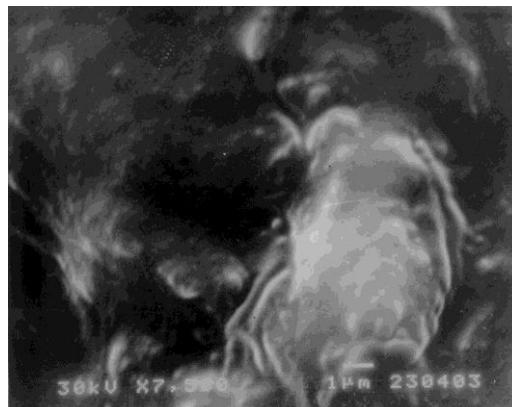
Figure 2 The SEM micrograph of NR/CSM/WRP composites filled with 20 phr waste rubber powder at 7500X magnification.
