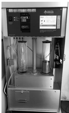
Figure 5. Gravimetric sampler of solid particles TSP, PM10 and PM2.5
