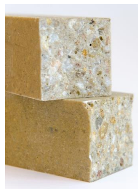
Figure 1. Cross-section of polymer-concrete product.
