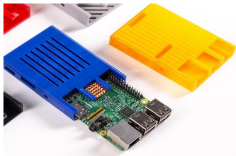
Figure 10. 3D printed cases for electronic devices based on PET-G.
