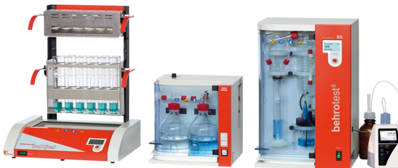
Figure 3. Apparatus for determining protein amount by the Kjeldahl method in flaxseed cake
