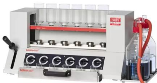
Figure 2. Apparatus for the determination of fibre content
