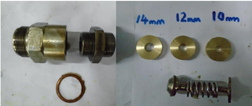
Figure 7 – Valve with a spring and calibrated orifice for regulating the fuel flow.
