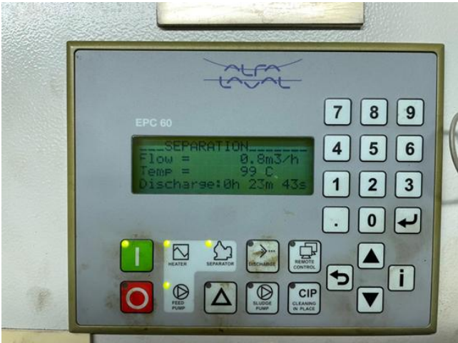
Figure 8 – Display of adjustable, maximally reduced flow through the fuel separator using calibrated orifice
