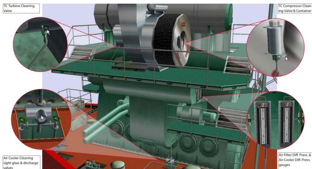
Figure 2. Turbocharger cleaning -compressor side (Transas Marine 2016 MAN B&W 6S60MC-C Diesel Engine – Tanker LCC. Trainee Manual pdf)
